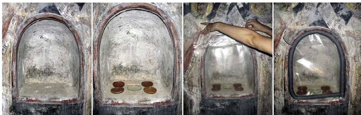
Figure 1. Ad-hoc-constructed aromatic chamber for in situ application of Boswellia carteri essential oil vapors aimed at cleansing fungal-contaminated air within the old Church of the Holy Ascension (Serbia).
